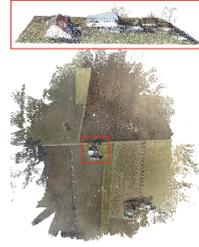
**Fig. 19.** Point-cloud generated by the RGB camera mounted on the FW-UAV. The house area shown in the top consists of 163'595 points.
