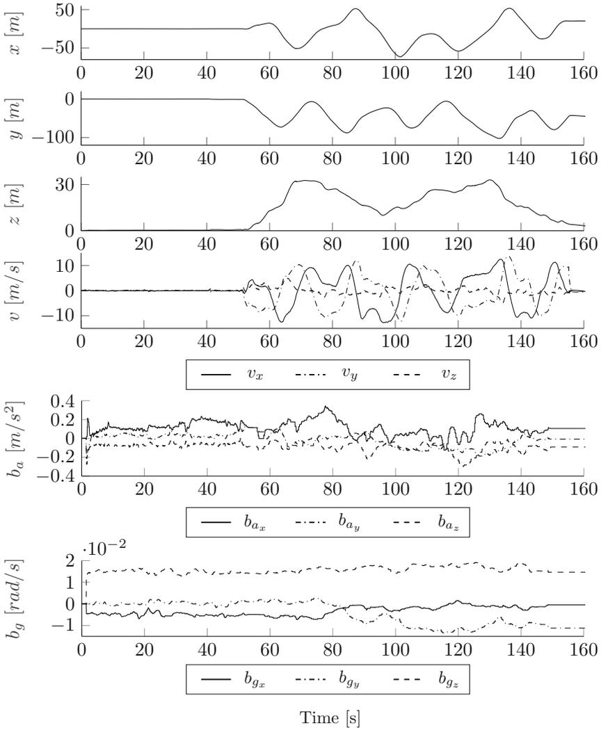
**Fig. 6.** State estimates of robot’s position, velocity, accelerometer as well as gyroscope biases.
