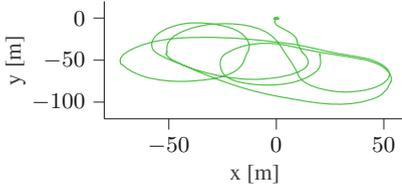
(a) Top-view of the estimated trajectory in local vision frame. The position is set to zero during initialization. The trajectory shows smooth estimates during take-off and landing phase.
