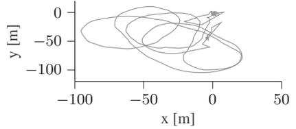
(b) Top-view of the GPS trajectory in local UTM coordinates where the first GPS measurement defines the origin. Especially at low altitudes, the GPS measurements show large jumps due to multi-path effects.
