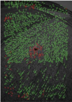
(a) The image visualizes the output of the vision front-end: Inlier feature tracks are shown in green. Tracks classified as outliers by RANSAC are visualized in red - here mainly due to the UAV's shadow violating the static feature assumption.
