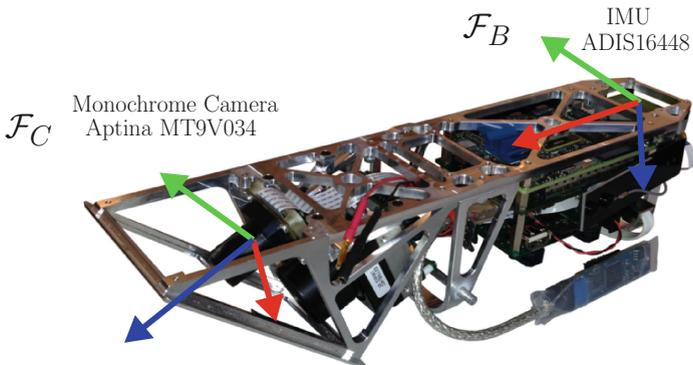
Fig. 1. Camera and body coordinate frame of the sensor processing unit.
