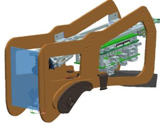
(b) CAD model of sensor & processing unit as well as its power interface to SKATE. The sensors consist of an IMU and a gray-scale camera.
