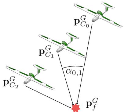
(b) Definition of well-constrained landmarks illustrated by the incident rays of three landmark observations. The following heuristics are used for the UAV SKATE datasets:  $M_{min} = 30$ ,  $d_{min} = 0.1$  m,  $d_{max} = 100$  m,  $\alpha_{min} = 0.5$  deg.
