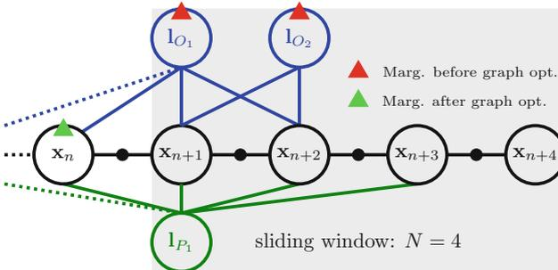
**Fig. 3.** Marginalization strategy: At step  $k = n + 3$  the VI-node is propagated and the graph is augmented with the new state  $\mathbf{x}_{n+4}$ . Due to the temporal condition (TC) the value node  $\mathbf{x}_n$  is to be marginalized. Also, the opportunistic landmark nodes  $l_{O_1}$  (TC) and  $l_{O_2}$  (not re-detected) are to be marginalized.
