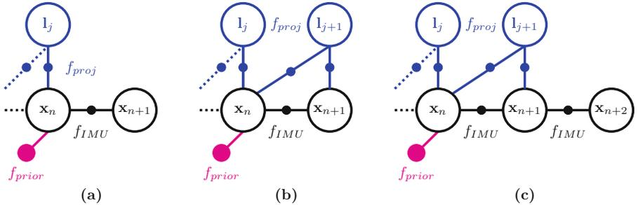
**Fig. 4.** Factor and value node insertion into the factor graph. (a) Initial setup at  $k = n+1$ . (b) Insertion of landmark values and reprojection factors. (c) Pre-integration of IMU measurements and graph augmentation.
