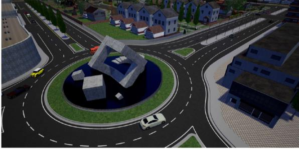
Fig. 7. A traffic circle in the CARLA simulator. We used CARLA to test more complex road topologies than were available at our test site.
