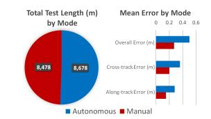
Fig. 9. A comparison of the LGPR estimates compared to ground truth in manual and autonomous driving modes.
