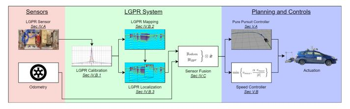
Fig. 4. The autonomous navigation pipeline which processed sensor inputs from the wheel odometry, and LGPR sensor, and computed steering and speed commands to send to the vehicle to autonomously drive the vehicle along the goal path.
