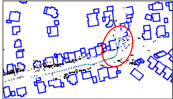
Fig. 6: Example of failed case. Accumulated drift in previous long straight road exceeds the range that the prior constraint could correct and hence wrong association is made leading to low tracking accuracy.
